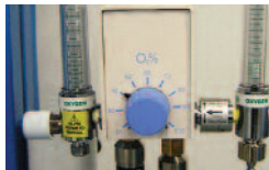
Air/O 2 Blender (PN 12368A70) It allows having a settable percentage O 2 on two outputs with different flow rates: 3 l/min or 15 l/min
