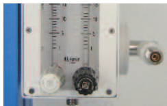
AIR O 2 / MIXER (PN 12432A70) It allows setting flow rate and percentage of O 2 by adjusting the inputs according to the corresponding table. It is possible to have an output with only Air, O 2 or both and the other one with Vacuos.
